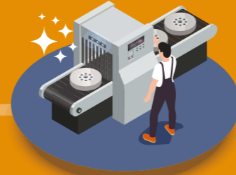
ROBOTISED DEGREASING OF THE WHEEL HUB
